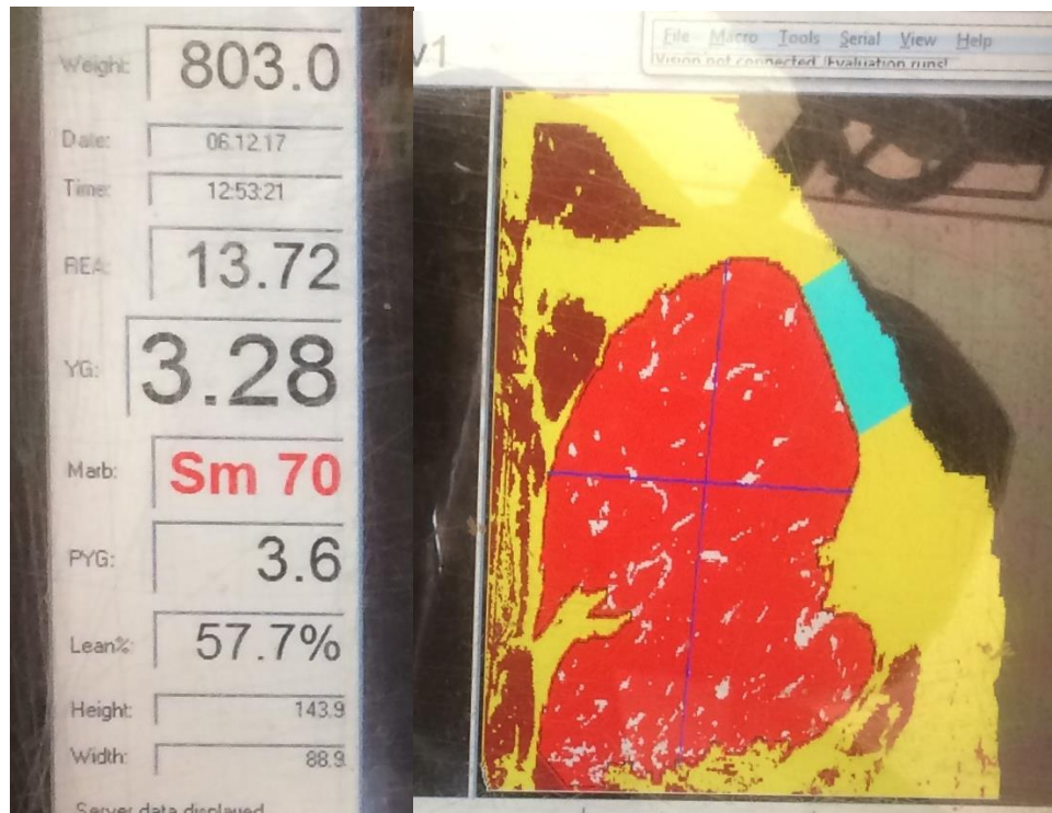
Figure 8 Electronic Image Analysis of REA
