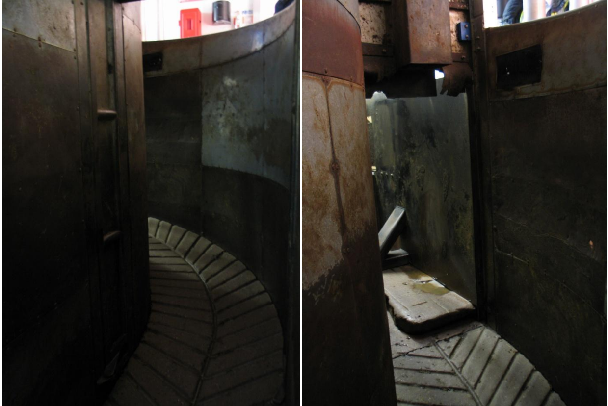
Figure 2. Original race and stun box conditions; light levels 5-35 lux in the race and 10-70 lux in the stun box.
