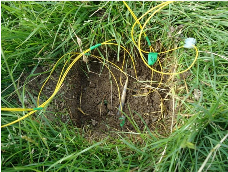
Figure 5. \text{NO}_3^- ISEs deployed in situ for field testing. The cut turf was replaced to ensure the \text{NO}_3^- ISEs were completely buried (Article IV)
